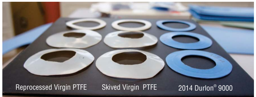
3D view of samples show a lot of distortion and warping with non-filled PTFE when compared with Durlon® 9000 samples.
