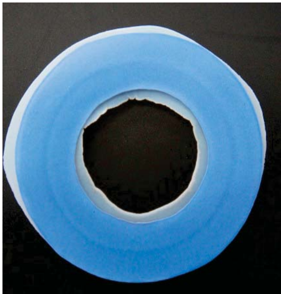
Overlay of Durlon® 9000 sample with Virgin Skived PTFE – Post Hot Compression Test
